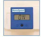
3. Turn on the cube reader by pressing the black button. After a brief period of self-testing, during which the reader shows WAIT, the reader will show ON. Press the black button.
