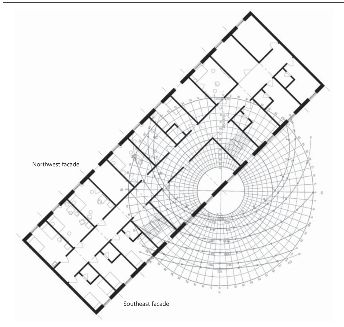
Fig. 2. Orientation of individual rooms.
