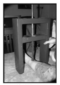
Fig. 1. Apparatus used for tibial tenderness measurement. This metal instrument with a rubber head was designed to apply 1 kg of weight to a 1-cm<sup>2</sup> area.
