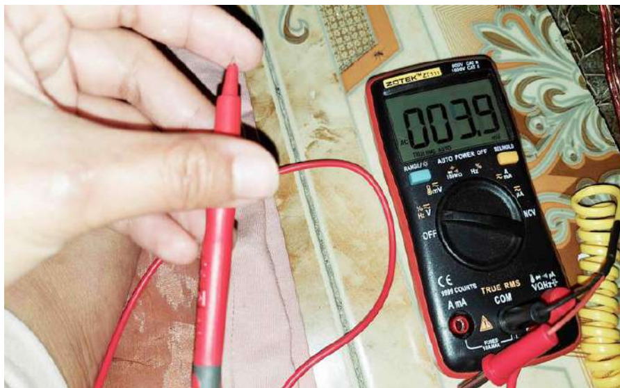
Figure 6. Measurement of skin voltage using Earthing device fluctuates between 3.9 mV up to 0.0 mV Picture source by Estiningtyas
