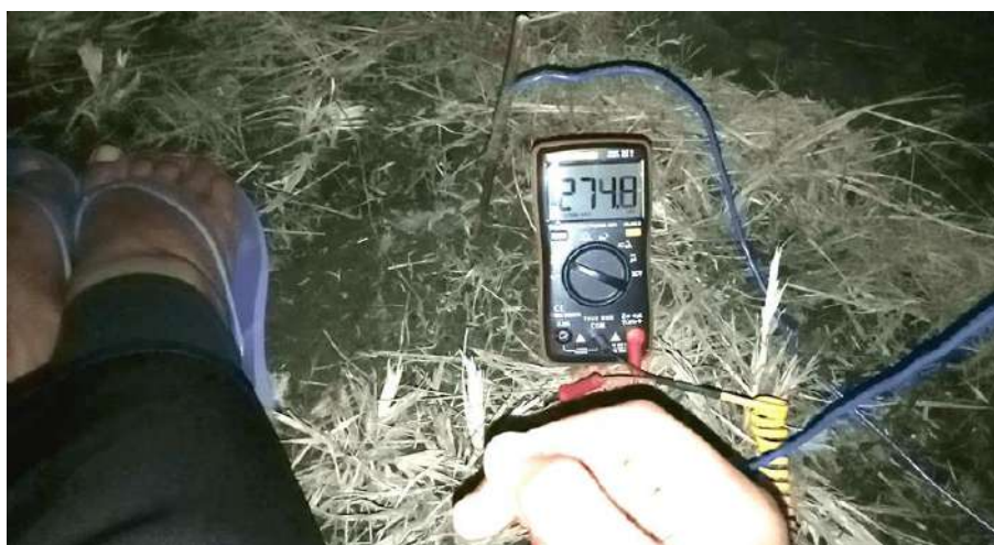
Figure 3. Skin voltage measurement before grounding results in 274.8 mV Picture source by Estiningtyas
