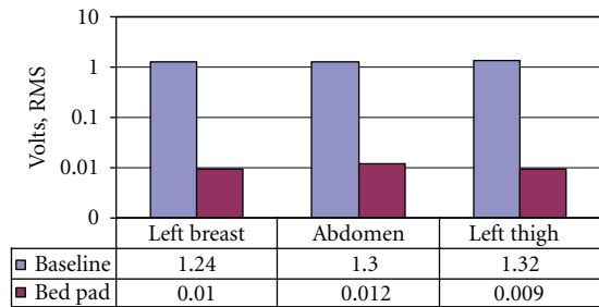
FIGURE 2: Effect of bed pad grounding on 60 Hz mode.
