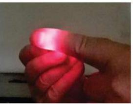
FIG. The penetration depth of light is determined by wavelength, not optical power
