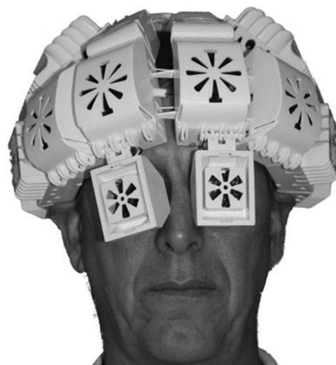
FIG. 1. The 1068 nm LED helmet showing positions of the LED modules. LED, light emitting diode.
