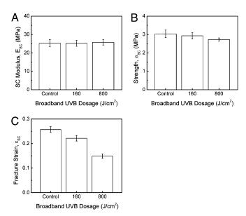
**Fig. 2.** (*A*) SC modulus, (*B*) SC fracture strength, and (*C*) SC fracture strain as a function of UV treatment for samples exposed to dosages of 0, 160, and 800 J/cm<sup>2</sup> UVB broadband radiation.
