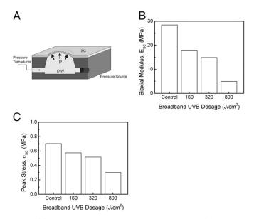
**Fig. 3.** (*A*) Bulge specimen geometry and testing schematic, (*B*) SC biaxial modulus, and (C) SC peak stress as a function of UV treatment for samples exposed to 160, 320, and 800 J/cm<sup>2</sup> UVB broadband radiation.
