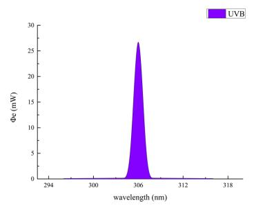
Figure 2. Spectrogram of ultraviolet light-emitting diode light. UVB: B-wave ultraviolet.
