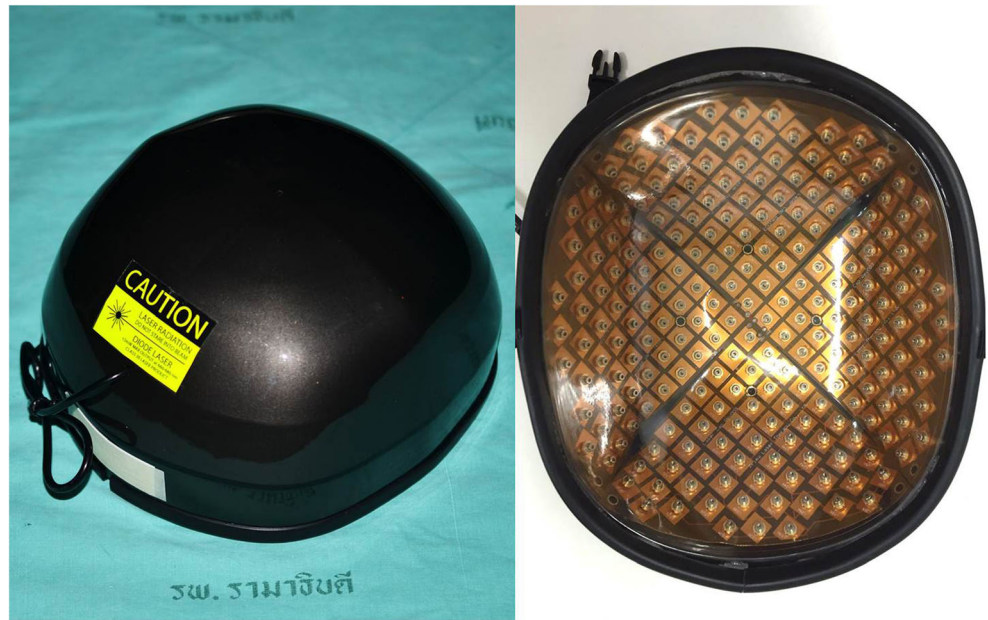
Fig. 1 RAMACAP, a helmet-type portable LLLT device containing 224 red diode laser bulbs (660 nm)
