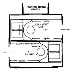
Fig. 2 .- Mounting of ultraviolet lamps in posts between cubicles.
