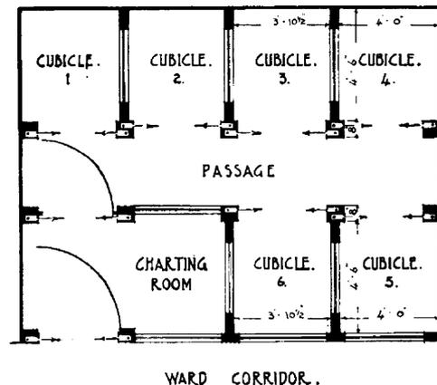
Fig. 1.—Plan of room equipped with ultraviolet lamps. Arrows show direction of ultraviolet rays.
