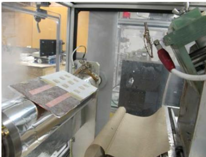
Figure 31: Kynurenine-loaded PVA on PLGA fibres in the fabrication of PLGA/PVA multi-layered fibrous structure
