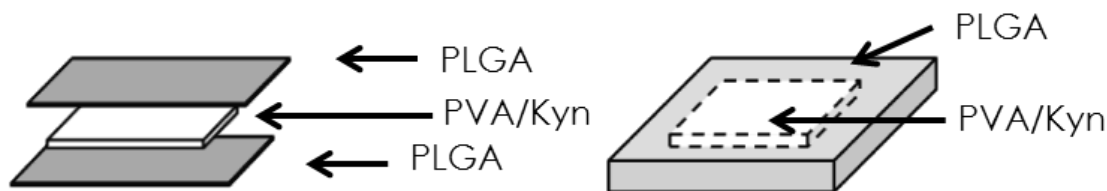
Figure 30: Graphical representation of the multilayer concept proposed in this thesis. The schematic on the left shows PVA/kynurenine nanofibres covered by PLGA nanofibre layers, whereas the schematic on the right shows PVA/kynurenine nanofibres dip-coated with PLGA
